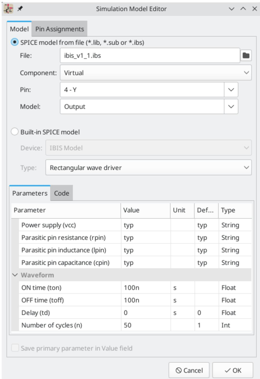
**File** is the path to the model file to use. The path can be absolute or relative to the project folder. The path can also be relative to the value of `SPICE_LIB_DIR` if you have [defined that path variable](#). The library filename is saved in the symbol's `Sim.Library` field. If an IBIS model file is loaded, the remaining fields in the dialog will relate to the IBIS model.
