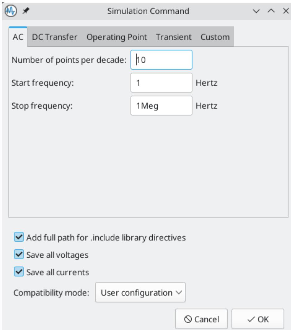
Calculates the small-signal AC behavior of the circuit in response to a stimulus. Performs a decade sweep of stimulus frequency.
