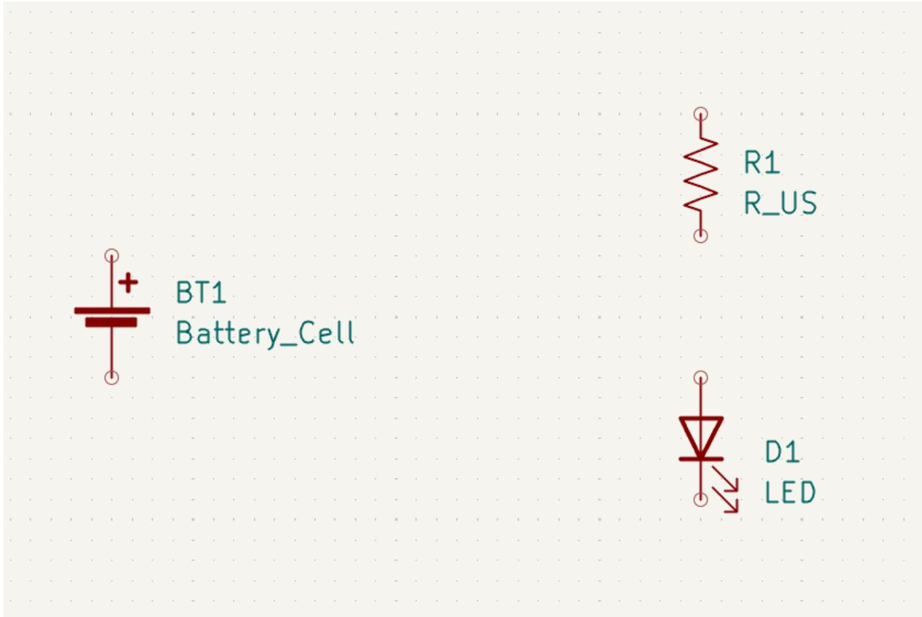
In KiCad, objects are selected by clicking on them while the selection tool is active. The selection tool is the default tool when no other tool is active, so you can enter the selection tool by quitting any active tool (`Esc`) or by clicking the button in the right toolbar.
